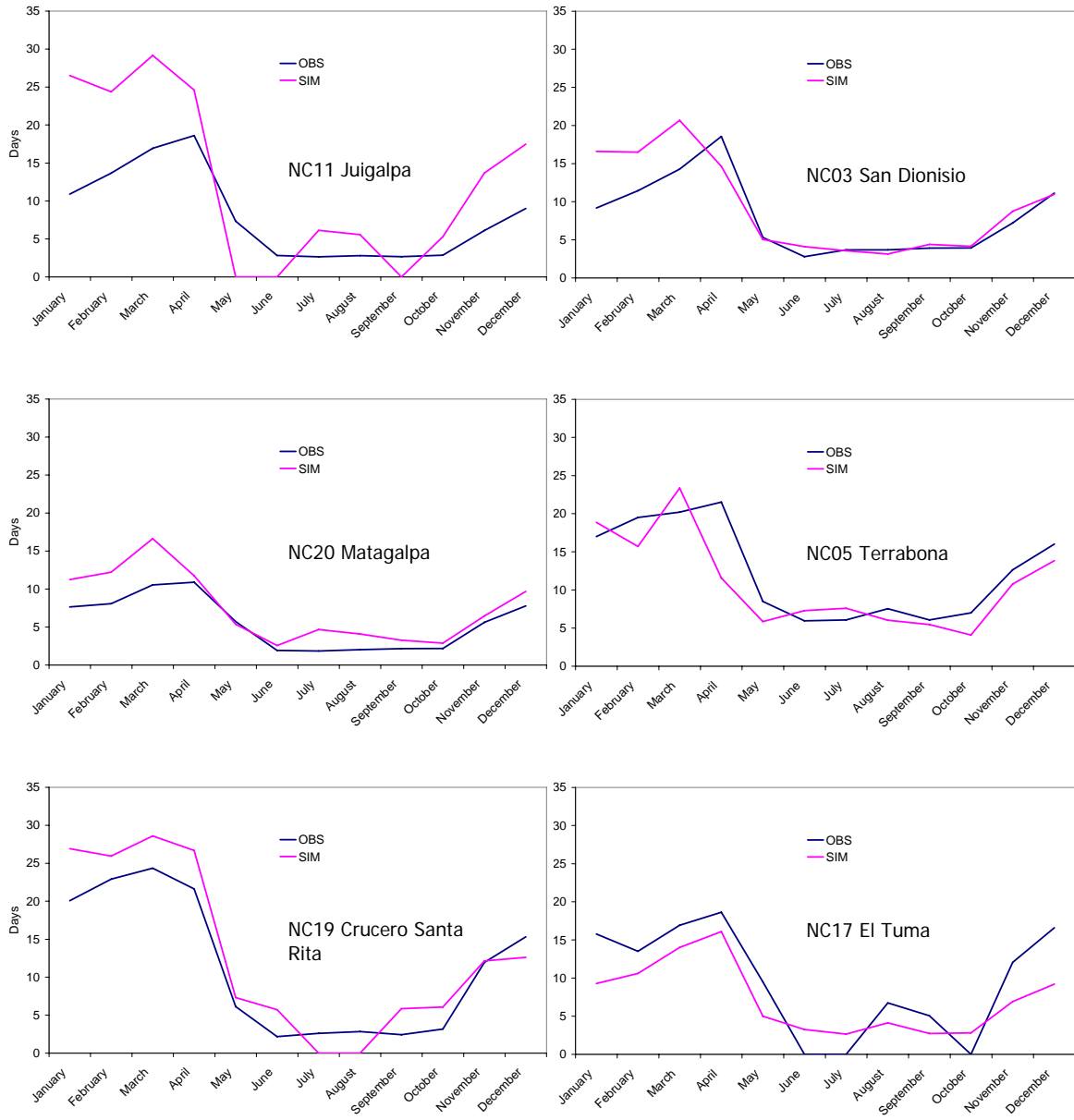
Figure 6-11 Average monthly length of dry spell length for the observed and simulated data sets. (continued).
